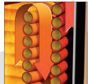
Heat is transferred to the thermal oil from all sides ensuring even heating
